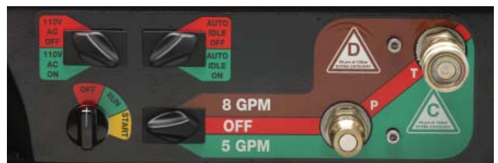
Figure 1. Panel Control Valve
